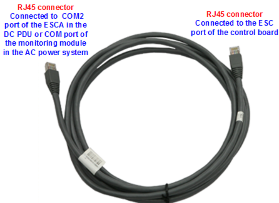
Figure 5-9 Appearance of a network cable
