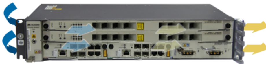
Figure 2-35 Ventilation of the MA5608T chassis
