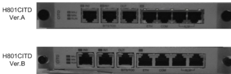
Figure 3-41 Differences in appearance between Ver.A and Ver.B
