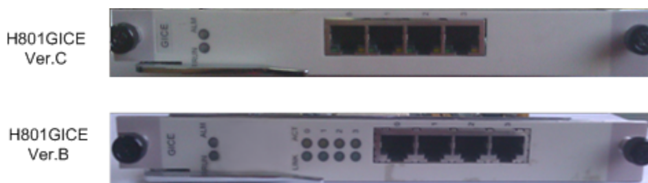
Figure 3-25 Differences in appearance between Ver.B and Ver.C
