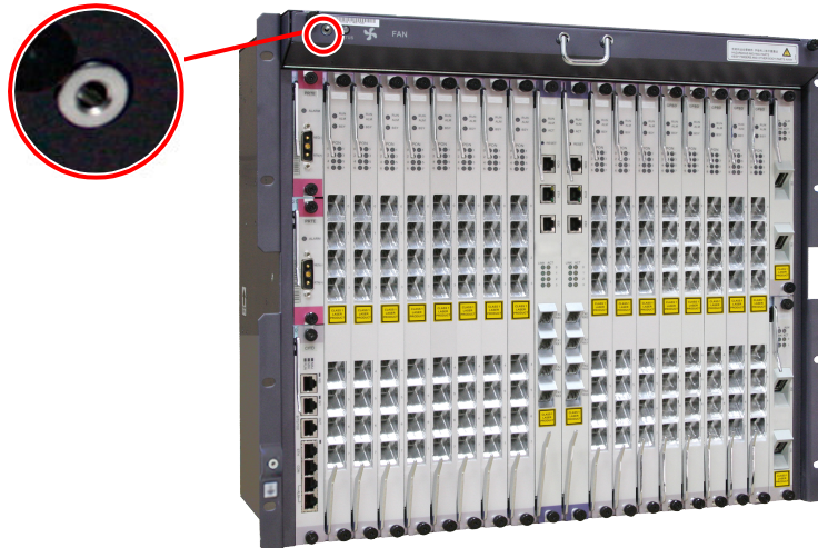
Figure 2-4 Position of the ETSI subrack ESD jack
