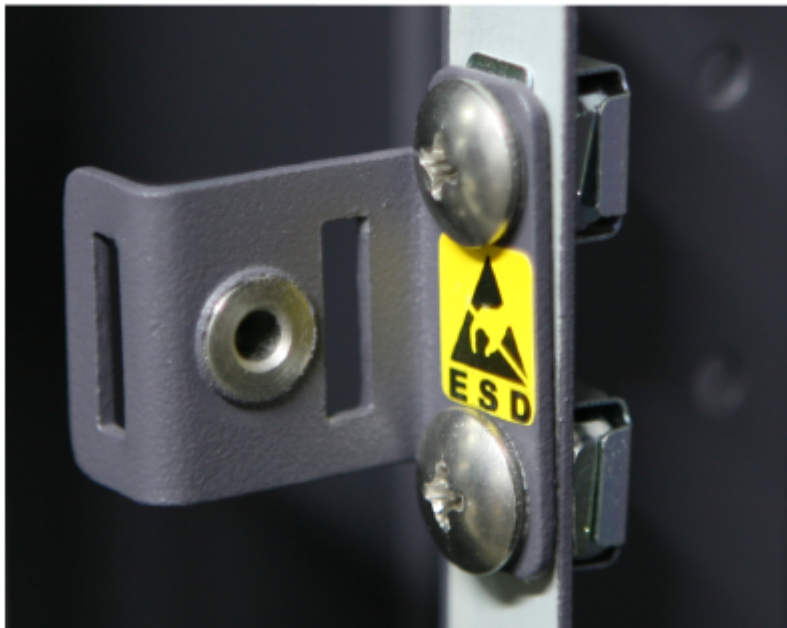
Figure 1-36 ESD jack of the N66E-18 dual-standard cabinet
