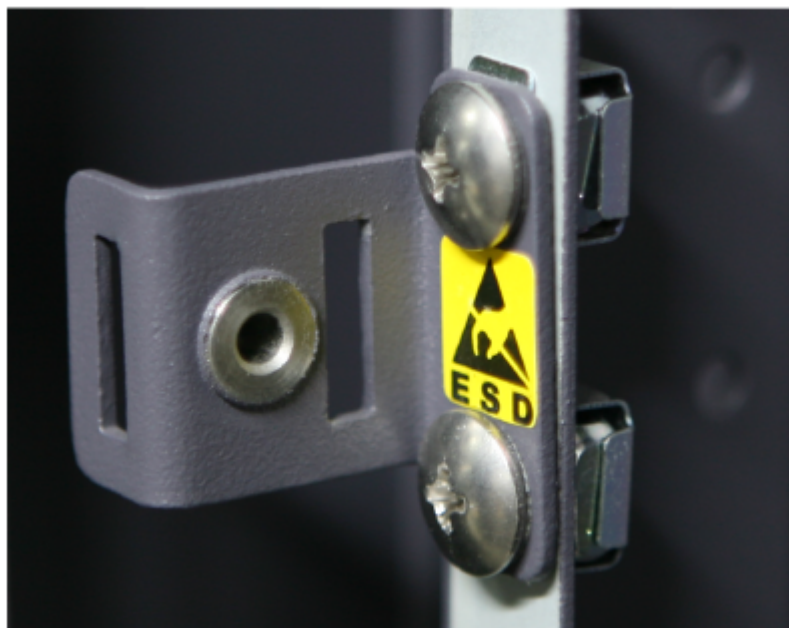
Figure 1-11 ESD jack of the N63E-22 cabinet
