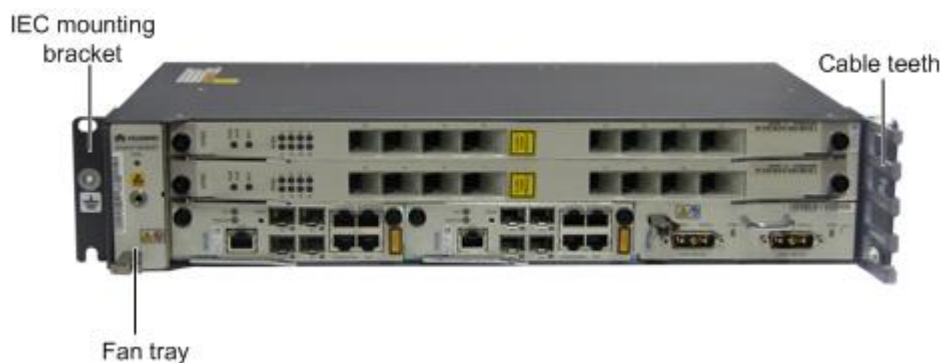
Figure 2-28 Appearance of the MA5608T chassis(GPON)
