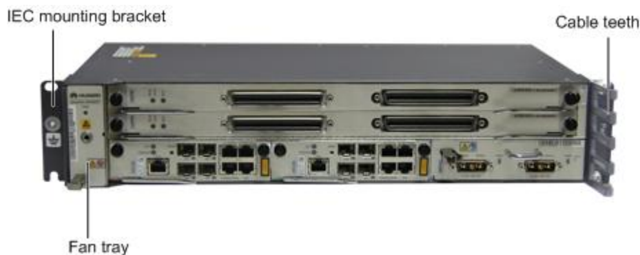
Figure 2-27 Appearance of the MA5608T chassis(xDSL)
