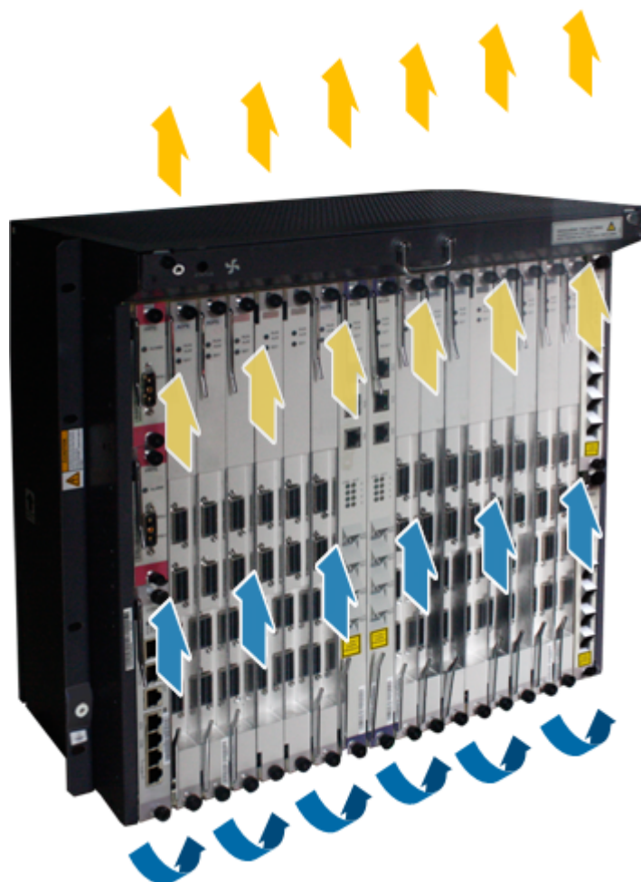
Figure 2-13 Ventilation of the MA5600T IEC service subrack
