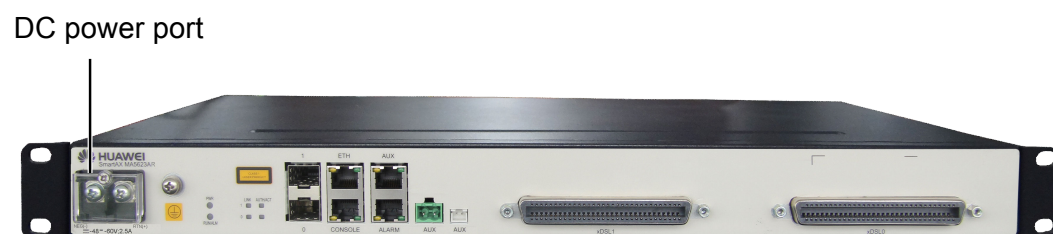
Figure 2-15 Appearance of an DC-powered MA5623AR
