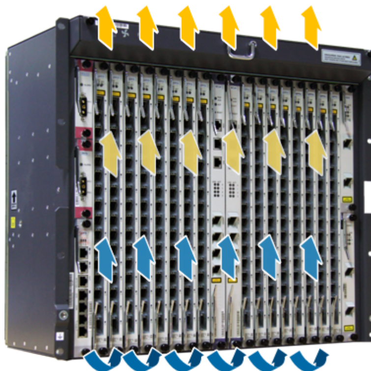
Figure 2-6 Ventilation of the MA5600T ETSI service subrack
