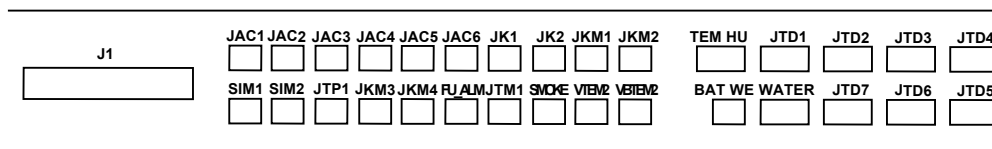
Figure 6-35 Sensor ports of the PMIB02 sensor transfer box
