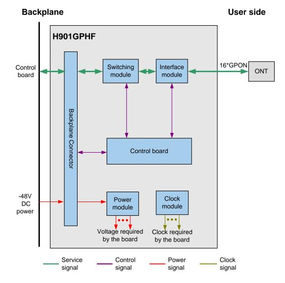
Figure 4-8 Working principle of the H901GPHF board
