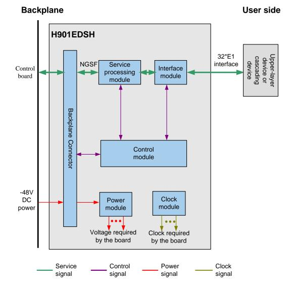
Figure 4-11 Working principle of the H901EDSH board
