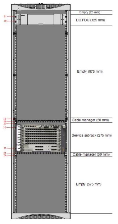
Figure 1-5 Configuration of the N63E-22 cabinet installed with one MA5800-X7 subrack
