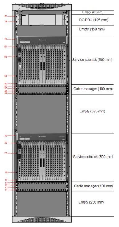
Figure 1-4 Configuration of the N63E-22 cabinet installed with two MA5800-X17 subracks
