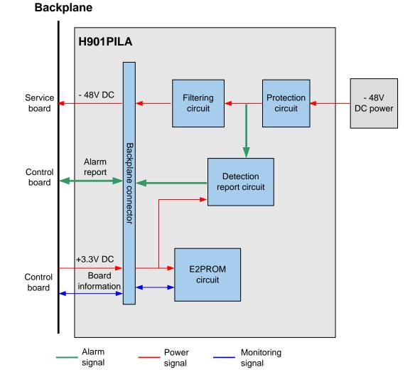
Figure 4-7 Working principle of the H901PILA board
