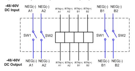
Figure 1-15 Diagram of the power distribution principle of the DPD60-4-4 DC PDU
