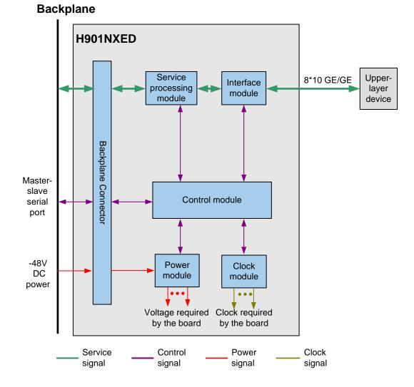
Figure 4-5 Working principles of the H901NXED board
