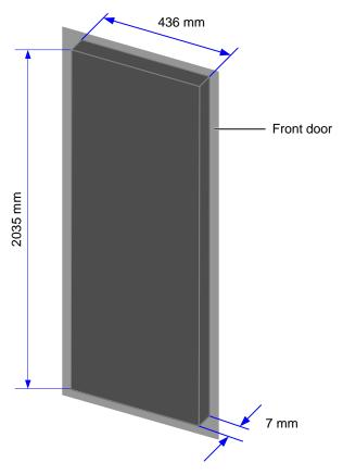
**Table 1-3** Material and dimensions of the air filter on the inner side of the front door of the N63E-22 cabinet
