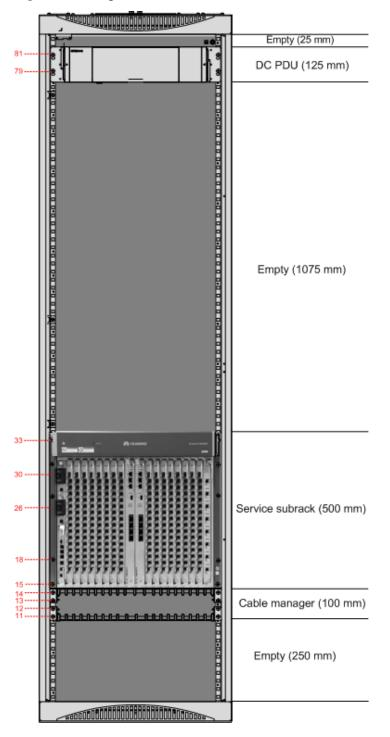
Figure 1-3 Configuration of the N63E-22 cabinet installed with one MA5800-X17 subrack
