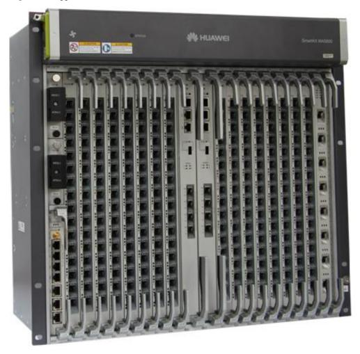
Figure 2-1 Appearance of the MA5800-X17 service subrack
