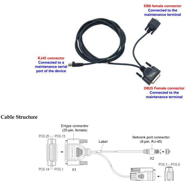
X3 D-type connector (9-pin, female) POS.5
