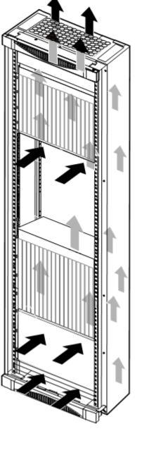
Figure 1-12 Ventilation of the N63E-22 cabinet installed with two service subracks
