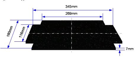
Figure 1-9 Appearance of the air filter at the bottom of the N63E-22 cabinet
