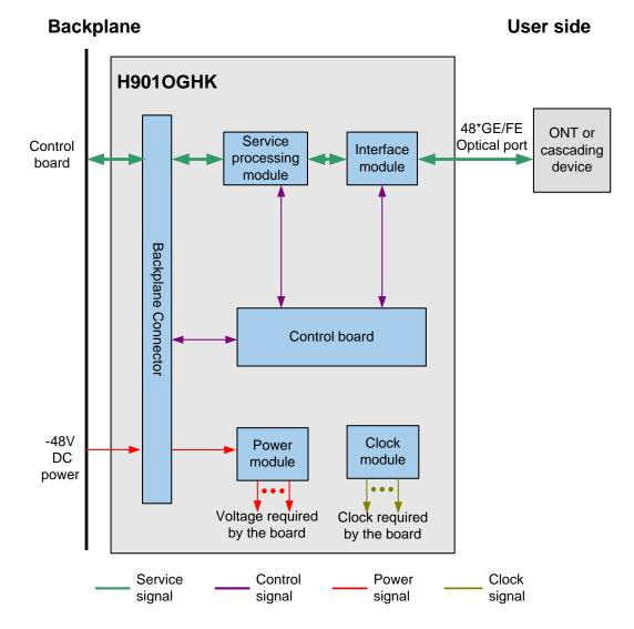
Figure 4-12 Working principle of the H901OGHK board
