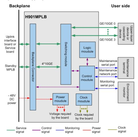
Figure 4-4 Working principle of the H901MPLB board
