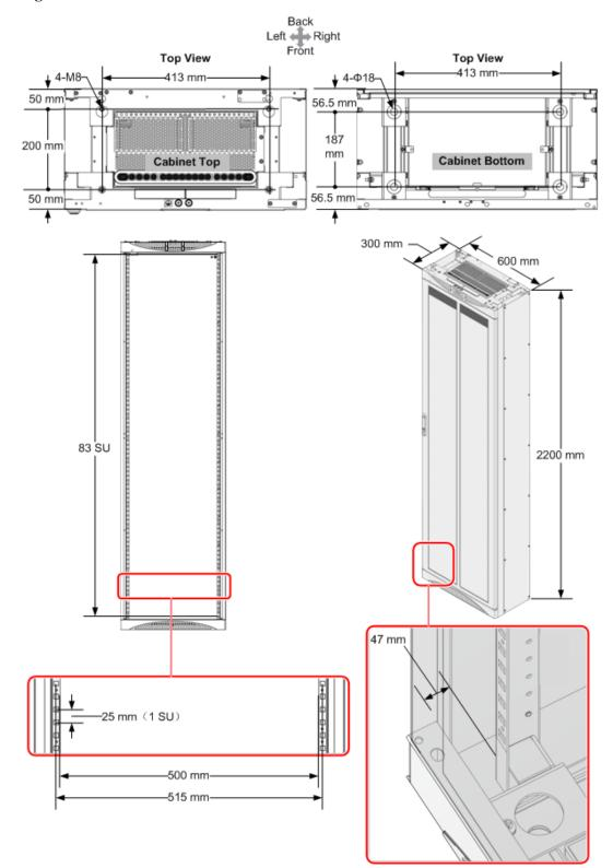
Figure 1-2 Dimensions of the N63E-22 cabinet
