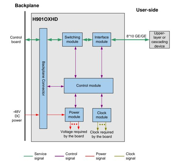
Figure 4-13 Working principle of the H901OXHD board
