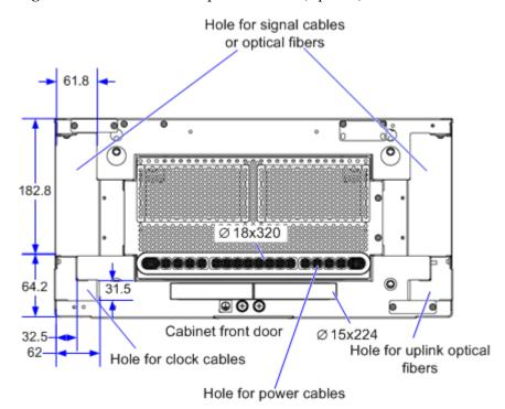
Figure 1-6 Cable holes at the top of the cabinet (top view)
