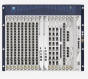
ZXA10 C600 is 11U high optical access equipment, which has 17/15 line card slots and can support 272/240 GPON/10G PON ports
