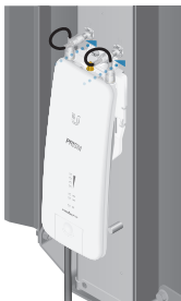
Connecting to a Sector Antenna
