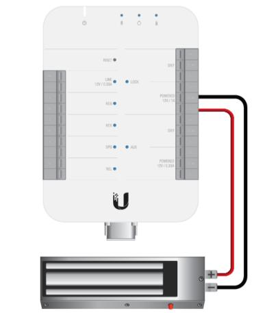
Connecting a Fail-Safe Lock with an External Power Supply
