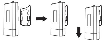
Installing the RocketM Titanium on an airMAX BaseStation or RocketDish antenna requires no special tools. You simply snap it securely into place with the universal Rocket mount built into the antennas.
