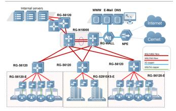
RG-S6120 can be deployed for the access or aggregation of small and medium campus networks. The 10G access ports can be used for high-speed AP access, forming 10G/25G access-to-aggregation and 40G aggregation-to-core high-bandwidth link to meet the users' growing needs.
