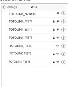
C. Launch a web browser from your smartphone. D. In the address bar, type the router's IP address 192.168.0.1, and then touch Enter. Enter the de-fault user name admin and password admin, and then touch LOGIN.
