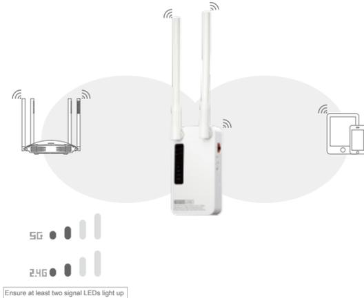
Ensure at least two signal LEDs light up
