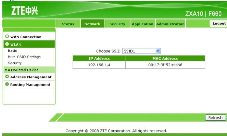
The screenshot shows the ZTE F660 web interface. The top navigation bar includes 'Status', 'Network', 'Security', 'Application', 'Administration', and 'Logout'. The 'Network' tab is selected, and the 'WLAN' sub-tab is active. Under 'WLAN', the 'Associated Device' option is selected. A dropdown menu for 'Choose SSID' is set to 'SSID1'. Below this, a table lists associated devices:
