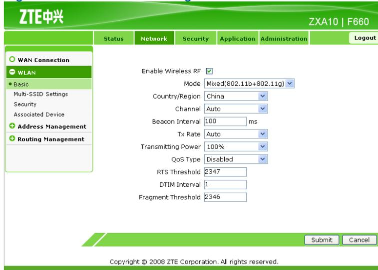
The screenshot shows the ZTE F660 Basic WLAN Configuration interface. The left sidebar contains a tree view with 'WLAN' selected and 'Basic' sub-selected. The main configuration area includes the following parameters:
