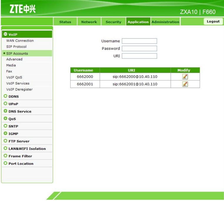
The screenshot shows the ZTE web interface for the ZXA10 F660 device. The 'Application' tab is selected, and the 'SIP Accounts' option is highlighted in the left-hand menu. The main content area contains three input fields: 'Username', 'Password', and 'URI'. Below these fields is a table listing existing SIP accounts.
