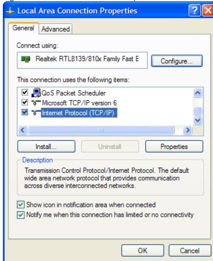
5. Click **Properties** to open the **Internet Protocol (TCP/IP) Properties** dialog box. Select **Use the following IP address** and specify the **IP address**, **Subnet mask**, and **Default gateway**. For example, you can set the **IP address** to 192.168.1.7, **Subnet mask** to 255.255.255.0, and **Default gateway** to 192.168.1.1, as shown in [Figure 8](#).
