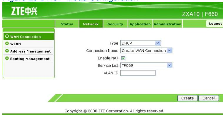
The screenshot shows the ZTE F660 web interface for DHCP mode configuration. The interface includes a navigation menu with options like WAN Connection, WLAN, Address Management, and Routing Management. The main configuration area shows the following settings:
