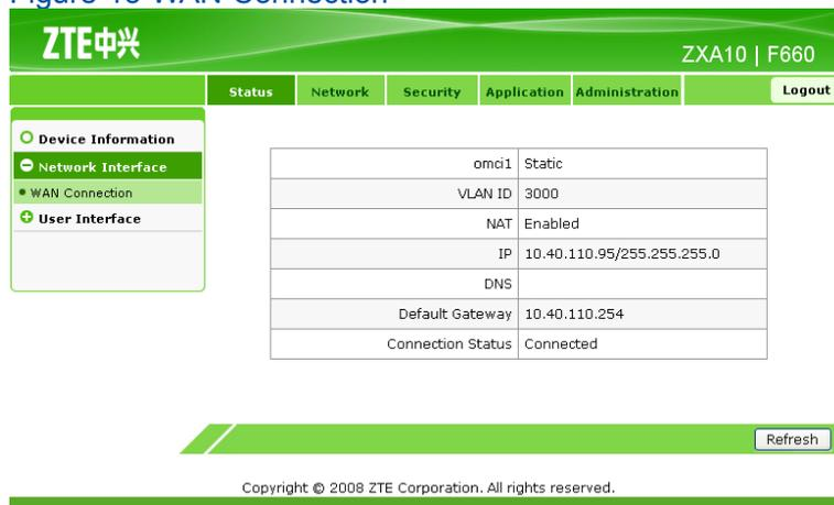
The screenshot shows the ZTE management interface for the ZXA10 F660. The 'Network Interface' section is active, and the 'WAN Connection' sub-tab is selected. The interface displays the following parameters:
