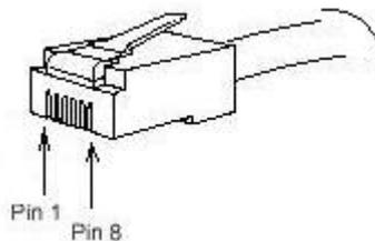
Figure 3-9 RJ-45 connector of the console port
